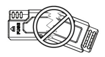
•Please do not bend the in-line control unit on the harness kit, it might cause the unit broken.
