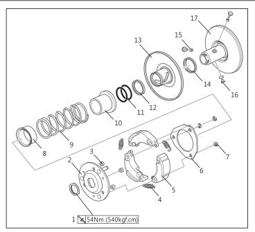
NOTE Please do according to figure in order. Make sure to disassemble the parts in reverse order. Please refer to the above picture for installation sequence.
