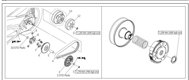
**NOTE** Please do according to figure in order. Make sure to disassemble the parts in reverse order. Please refer to the above picture for installation sequence.
