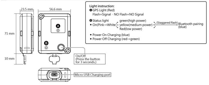
● USB charging voltageDC 5 V● Effective temperature range-10 ~ 60 °C● IP LevelIP54● Size71 X 56.6 X 23.5 mm● WeightAbout 75.5 g
