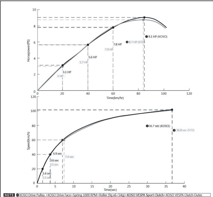
NOTE 2 KOSO Drive Pulley +KOSO Drive Face+Spring 1000 RPM+Roller (9g x6=54g)+STD VESPA Clutch+STD VESPA Clutch Outer.
