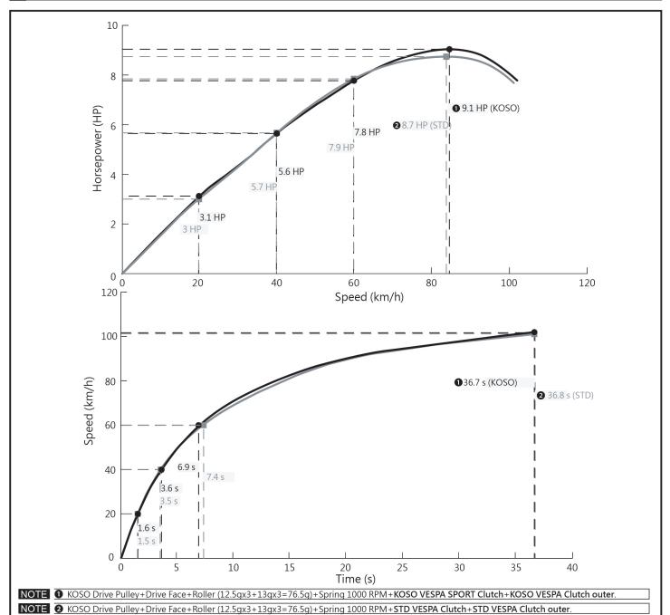
NOTE Test results vary with testing environment and weather. This test chart is for reference only.
