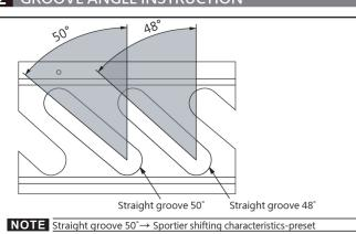
NOTE Straight groove 48°→Softer shifting characteristics-close to the original
