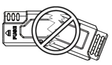
•Please do not bend the in-line control unit on the harness kit, it might cause the unit broken.
