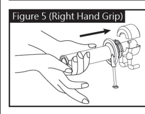
Insert throttle adaptor as well as grip to right hand handlebar.
