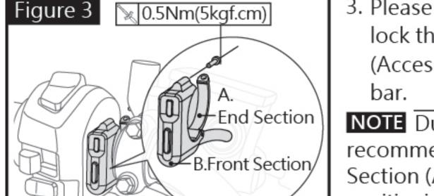
3. Please use proper tools to lock the CNC 5 Level Switch (Accessory 9) onto the handel
