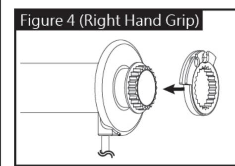
4. Use appropriate throttle adaptor (Accessory 5~7), and install the throttle adaptor according to the correct angle of the bike.
