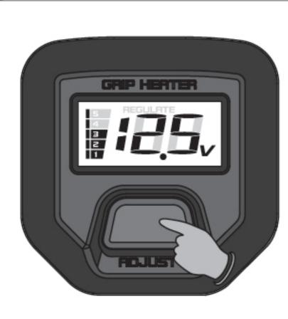
EX: Screen of 3rd of heating section. In main screen, press the button for 3
