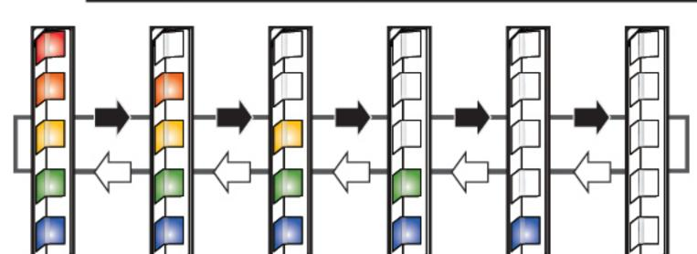
When the button remained idle for 5 seconds, the stage shifting will start from red LED light (stage 5) after pressing the button.
