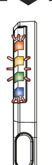
The corresponding light signal would be shown according to the power pressure detected.
