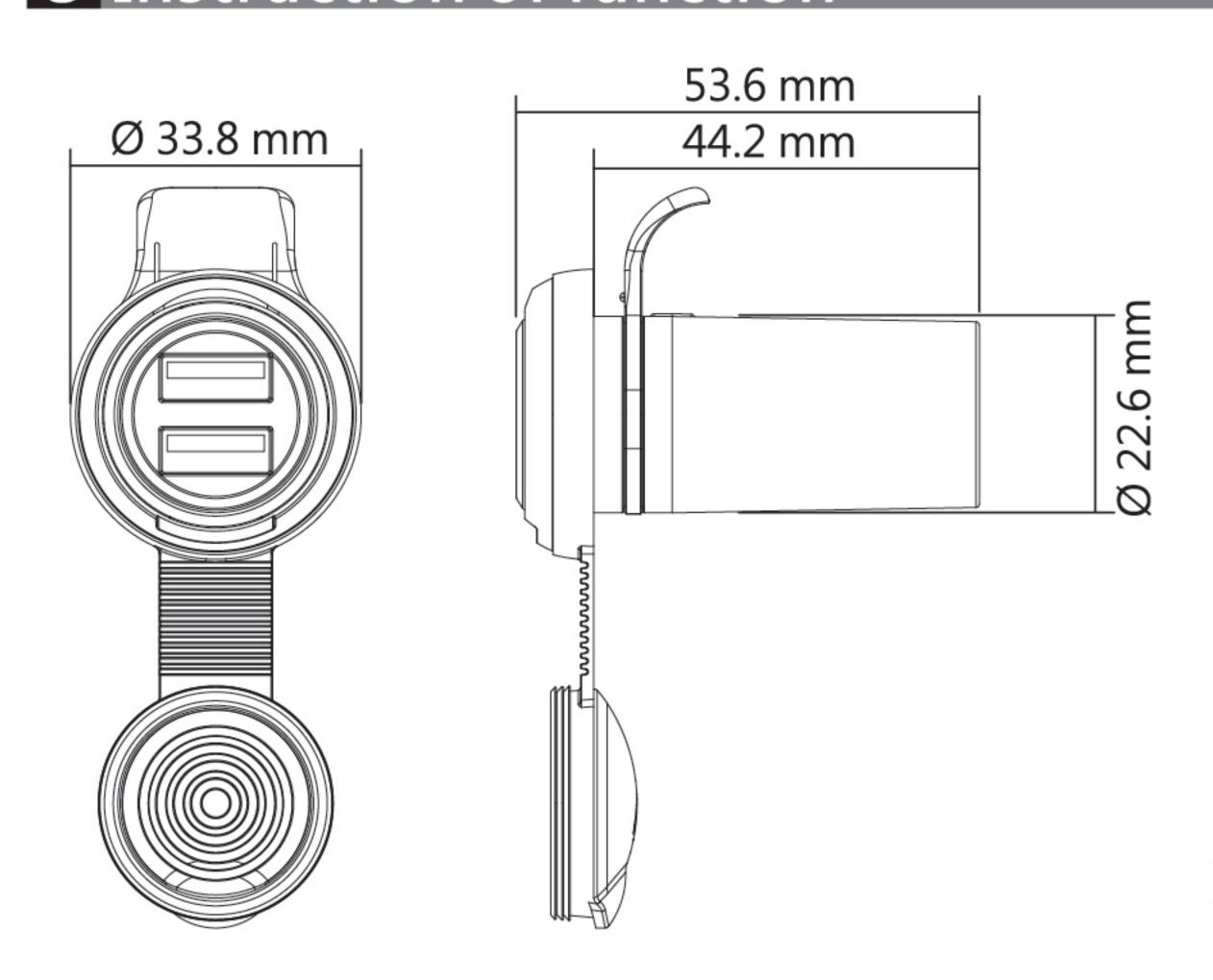
USB Working Voltage Voltage Range: DC 12.5 ~ 24 V
