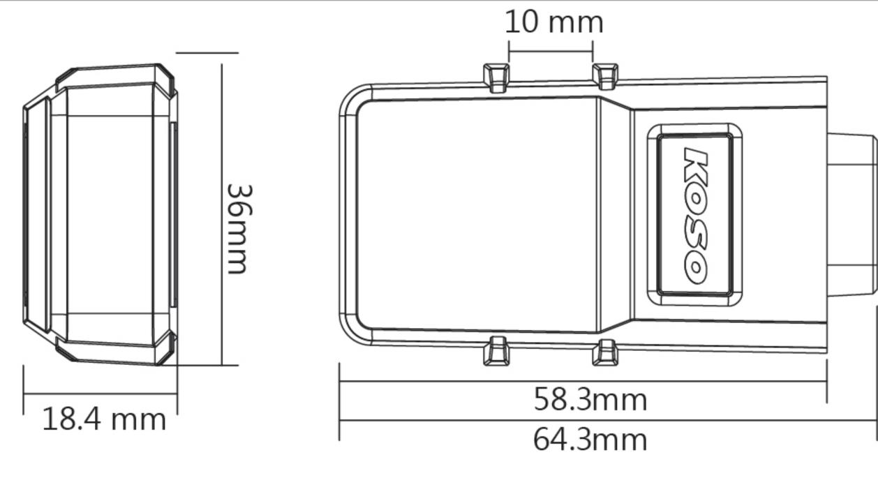
●USB Working Voltage Voltage Range: DC 11.5 ~ 16 V
