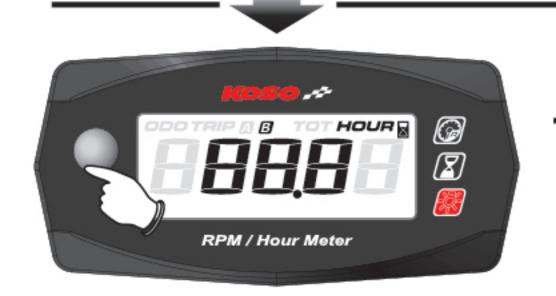
In the hour meter B screen, **press the button** one time to enter the RPM.
