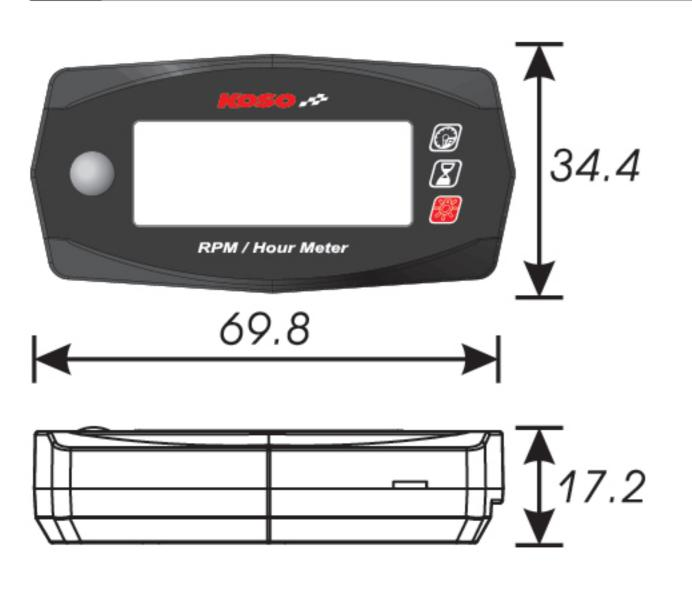
Digital Tachometer Display range: 0~15,000 RPM Display unit: 10 RPM ODisplay internal <0.5 Sec. ○MAX RPM record Display range:  $0\sim15,000$  RPM Setting range: 0.5, 1, 1.5, 2, 2.5, 3, 4, 5, 6 RPM input pulse Display range : 0~99999 H ■Total engine hour meter Display unit: 1 H ■Hour meter A/B Display range : 0.0~999.9 H Display unit : 0.1 H
