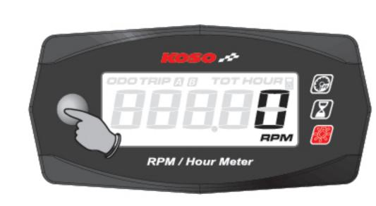
In RPM screen, hold pressing down the button for 3 seconds to enter the RPM pulse setting.
