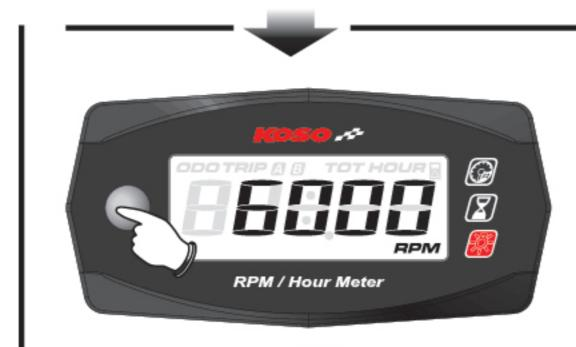
In the RPM screen, **press the button one** time to enter the Max. RPM record.
