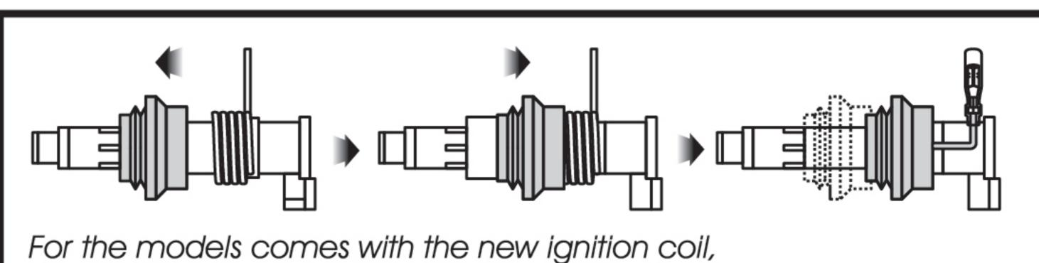
For the models comes with the new ignition coil, please wrap the RPM wire st least 5 times around the spark plug as the above drawing.
