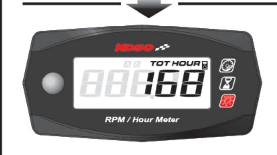
NOTE The meter will turn off automatically if you don't press the button or there is no signal input for 30 seconds.
