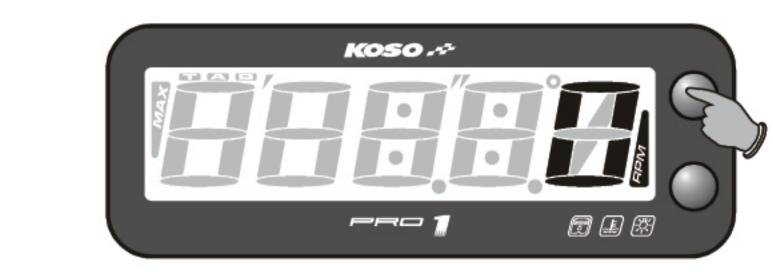
In RPM screen, Hold pressing the Select button for 3 seconds to switch function from RPM to thermometer.
