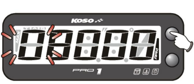
EX: You want the shift light to light on at 8000 RPM Please change the shift light setting value to 8500 directly.
