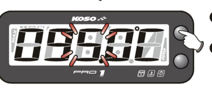
Press the Select button to go back to the temperature alarm screen.
