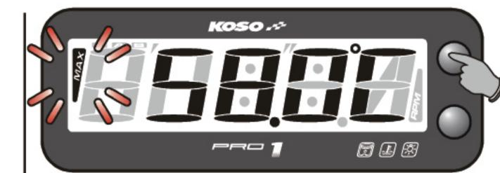
In MAX temperature record screen, Hold pressing the Select button for 3 seconds to go back to the RPM screen.
