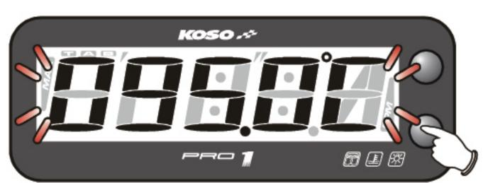
Press the Adjust button to enter the Backlight setting.
