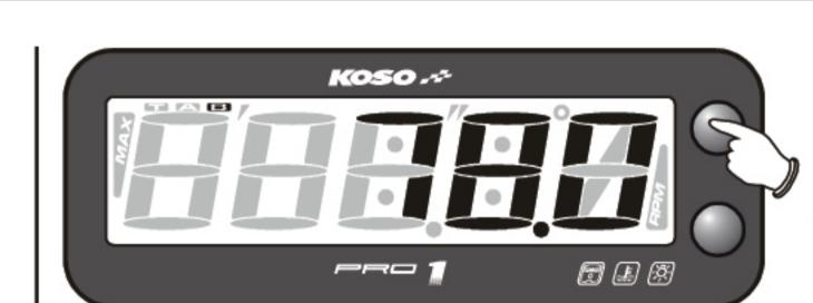
In hour meter B screen, Press the Select button once to switch function from hour meter B to MAX.
