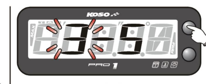
Press the Select button one time to enter the backlight setting.
