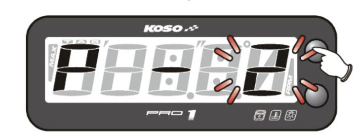
Press the Select button to go back to the RPM pulse setting.
