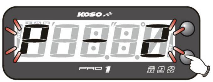
Press the Adjust button to enter the shift light setting.
