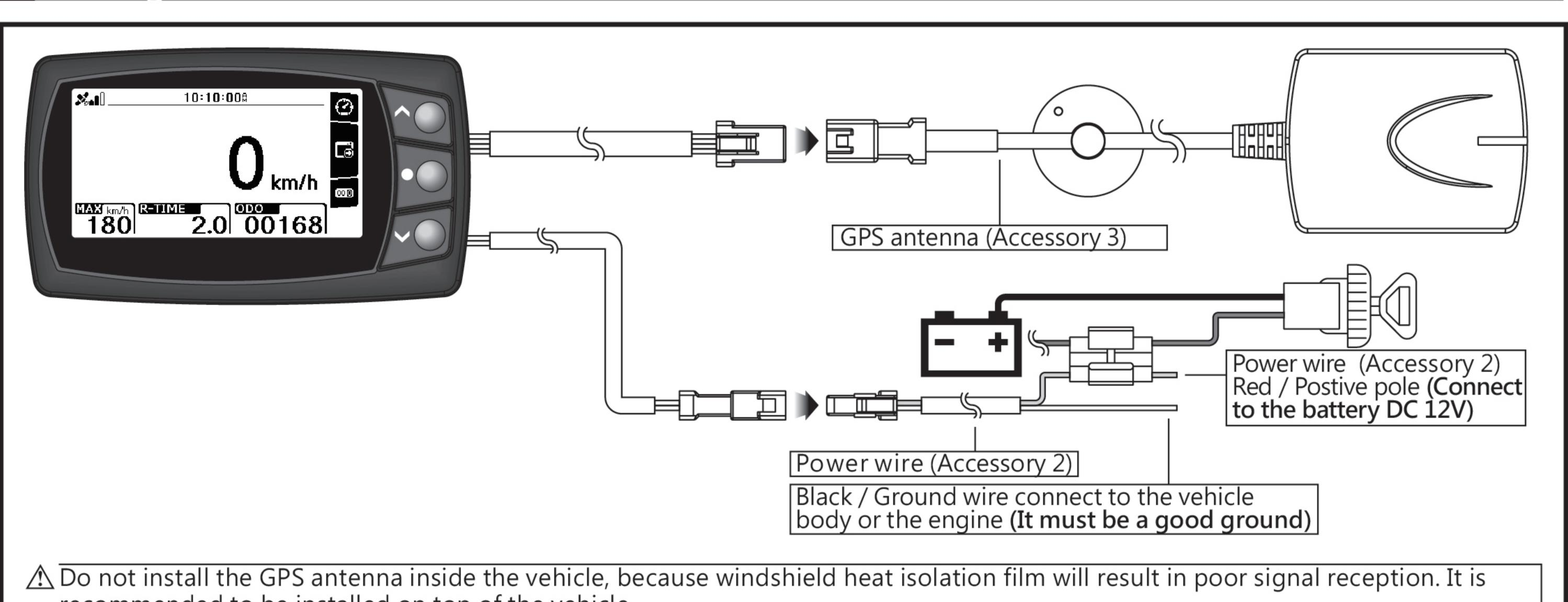
recommended to be installed on top of the vehicle.
