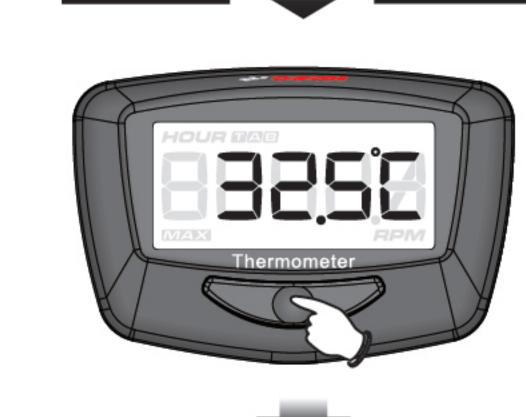
In temperature display screen, press the **button once** to enter the Max. temperature record screen.
