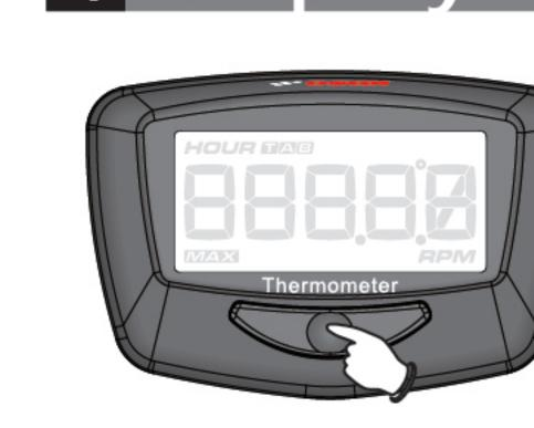
When meter is OFF, press the button once to enter the temperature display screen.
