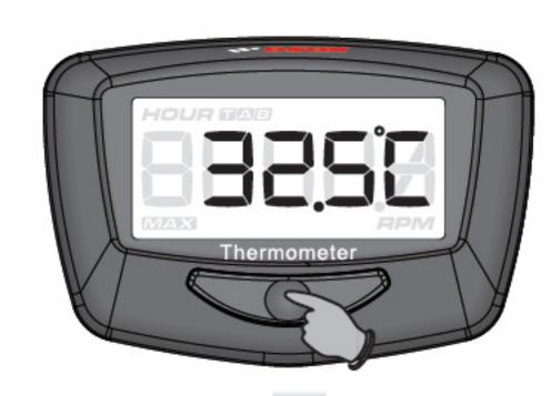
• In temperature display screen, press and hold the button for 3 seconds to enter the temperature unit setting.
