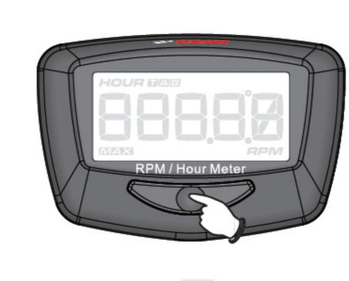
When meter is OFF, press the button once to enter the RPM display screen.
