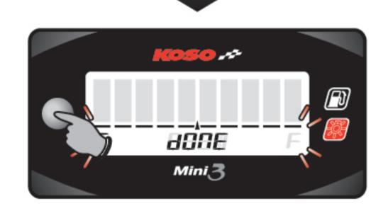
Hold pressing the button for 3 seconds to enter the full fuel setting screen.
