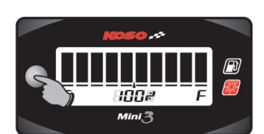
In main screen, Hold pressing the button for 3 seconds to enter the setting screen.
