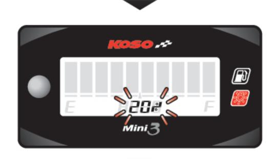
Hold pressing the button for 3 seconds to go back to the main screen.
