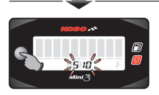
Hold pressing the **button for 3 seconds** to enter the fuel warning setting screen.
