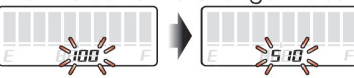
**NOTE** The fuel gauge resistance setting range:  $100\Omega$ ,  $180\Omega$ ,  $250\Omega$ ,  $270\Omega$ ,  $510\Omega$ ,  $700\Omega$ ,  $1200\Omega$ , USER.
