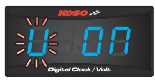
In turn on/off the volt warning screen, press the button for 3 seconds to enter the setting screen.
