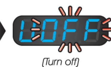
**NOTE** When setting is OFF, the voltage warning function is disabled. The high/low voltage warning will not be displayed.
