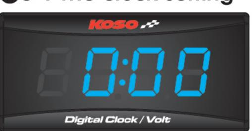
In the clock screen, press the button for 3 seconds to enter the clock setting screen.
