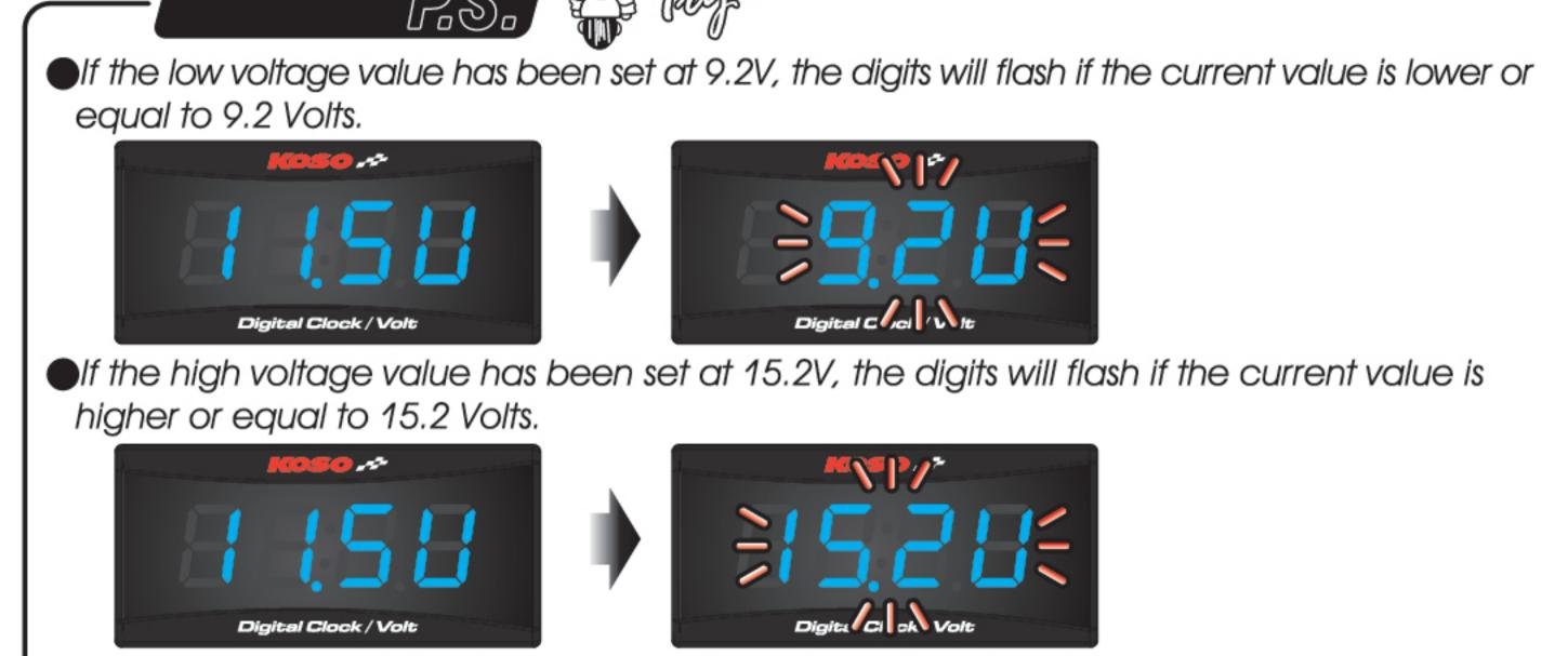
If the voltage reach the low or high setting, the meter will automatically switch to the voltage warning screen even if the meter is on the clock function.
