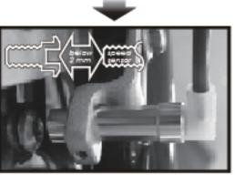
Adjusting the distance between the sensor and screw to get the best speed signal. Please make sure the distance is under **2 mm** to get the best signal.
