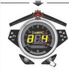
Press the Adjust button to enter next operation setting.
