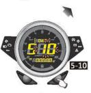
Press and hold the Adjust+Select buttons, and turn on the main switch until the boot animation ended and enter the basic function setting.
